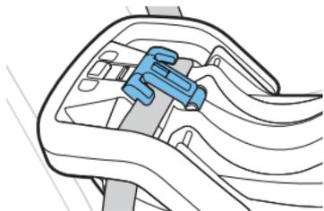
Lock-off must be used at all times when installing with a vehicle seat belt.
