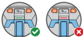
Ensure tightness indicator is **GREEN** after each use. If it is not, apply pressure by pushing base into seat bight (crease of seat) to tighten.
