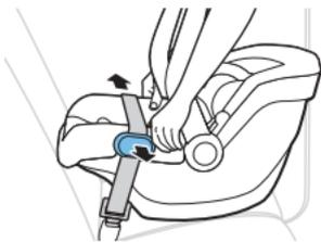
Carrier doesn't move more than 2.5 cm (1 in) side to side and more than 2.5 cm (1 in) front-to-back at the belt path.
