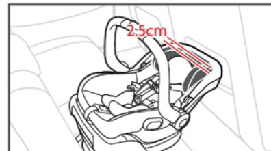
The top of the child's head should not be less than 2.5 cm (1 in) from the top of the headrest when in its highest position.
