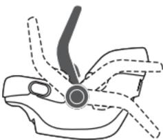
Move carry handle to the (3rd) carry position before removing carrier from vehicle.
