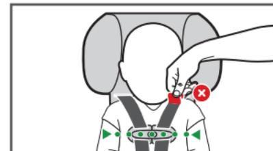
Retainer clip must be at armpit level **1** and harness straps should be snug **2**.
