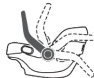
**NOTE:** The carry handle must be locked in the (4th) rebound position when in use.
