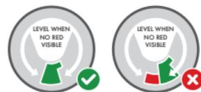
After attaching carrier to base check that the base is level. Base is level when only **GREEN** is visible between the two arrows on the level indicator.
