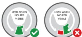
Recline angle is correct. Base is level when only **GREEN** is visible between the two arrows on the level indicator. No **RED** should be visible.
