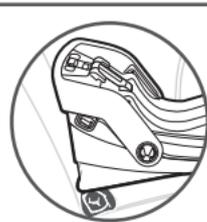
If proper angle cannot be achieved with adjustable foot, a rolled towel may be used. Foot must be in fully extended position.
