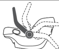
Carry handle must be locked in the (4th) rebound position when in use in the vehicle.
