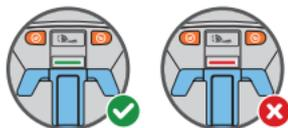
Ensure tightness indicator is **GREEN** after each use. If it is not, reinstall base.
