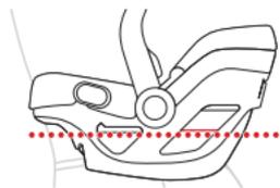
Angle is correct when The **RED** line on the carrier is level with the vehicle floor.
