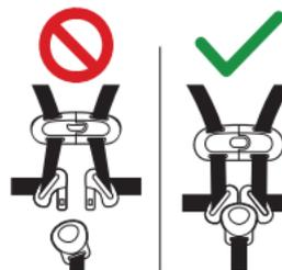
Children have **STRANGLED** in loose or partially buckled harness straps. Fully restrain the child even when carrier is used outside the vehicle.
