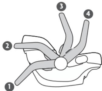
The carry handle must be locked in any four (4) positions when in use: stand ①, store ②, carry ③ and rebound (vehicle use) ④.
