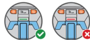
Push into the seat bight (crease of seat). Installation is complete when tightness indicator turns from **RED** to **GREEN** and stays green when downward push is discontinued.
