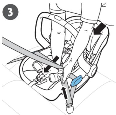
**⚠ WARNING!** Vehicle seat belt must lock, otherwise locking clip must be used. See page 49 for instructions.
