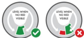
**NOTE:** Vehicle must be parked on a level surface to properly level the base.
