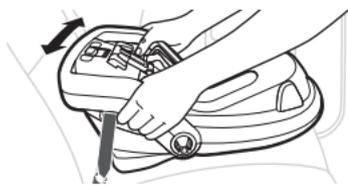
Base doesn't more than 2.5 cm (1 in) side-to-side and front-to-back at the belt path.
