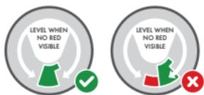
Recline angle is correct. Base is level when only **GREEN** is visible between the two arrows on the level indicator. No **RED** should be visible.
